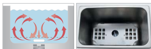
Powerful circulation by built in agitator
