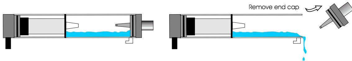
Carefully remove the end cap from the in-line housing. Dispose of the condensate in a suitable drain, care must be taken as it could be acidic. If condensate spills onto the skin or clothing, clean off immediately using fresh water, seek medical advice if problems occur.
