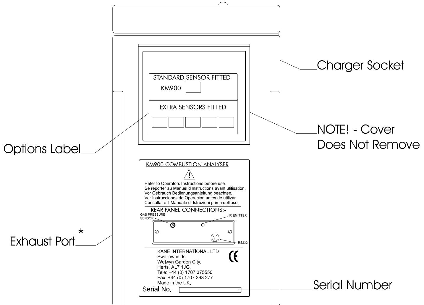
\*NOTE! Do not cover exhaust port as this will severely affect analyser operation
