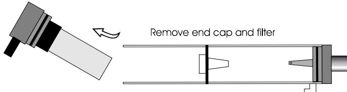
Remove the end cap from the in-line filter housing. Carefully remove the paper filter element and dispose of it. Clean the inside of the filter housing with a suitable soft cloth. Insert a new filter element onto the spigot in the filter housing and carefully replace the end cap.
