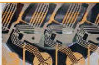
Sensor contacts: Au/Ni/CuFe
