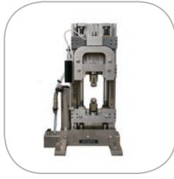
**MT2000ES** A stage designed specifically for EBSD applications in the SEM. Horizontal and 70 degree specimen clamps, available with fixed 1kN or 2kN loadcells and heating cooling options.
