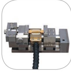
**CT500** A low load stage for cabinet based XRM ( $\mu$ XCT) systems with a polymer support tube holding the top jaws. Suitable for high resolution imaging of small samples under tension or compression.
