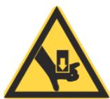
**This symbol is intended to alert the operator to the danger of crushing injury.**
