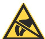
**This symbol is intended to alert the operator to the danger of Electro-Static Discharge (ESD) susceptibility.**
