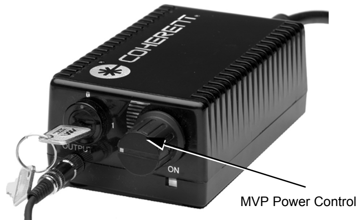
Figure 16. Laser Output Power Control
