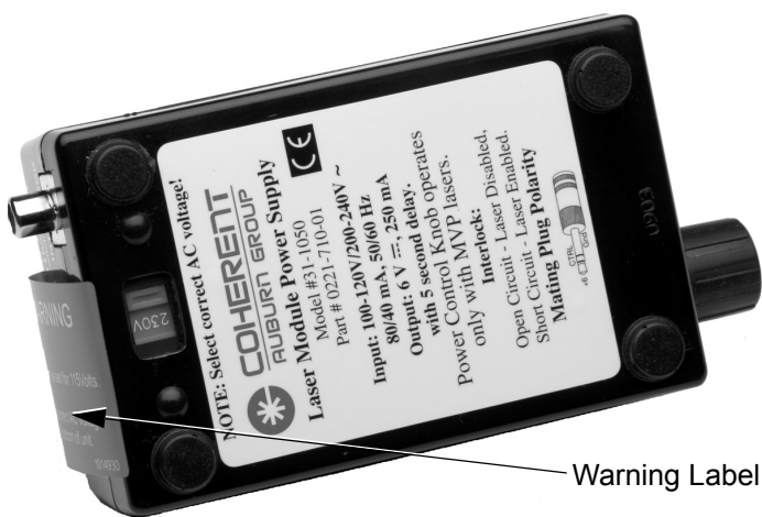
Figure 8. Voltage Warning Label
