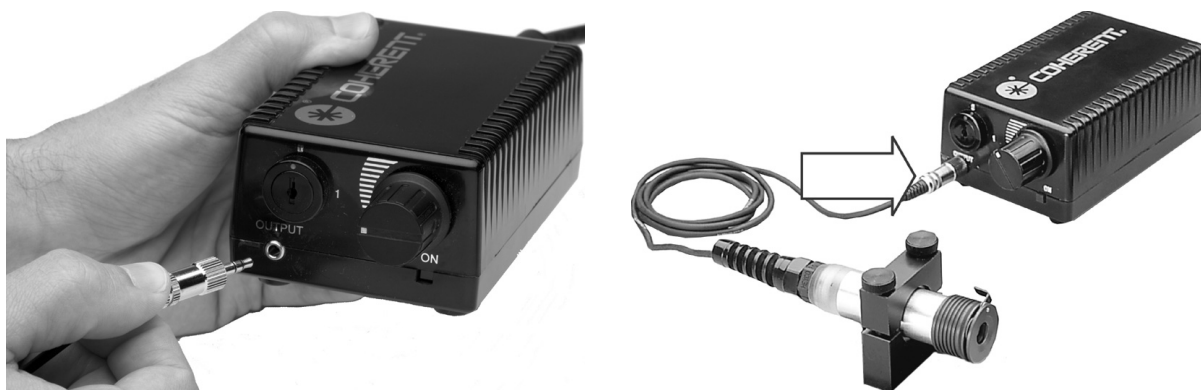
Figure 13. LabLaser Direction Connection to the Power Supply
