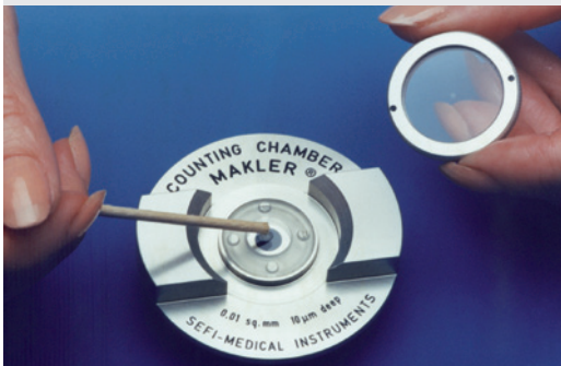
MAKLER Counting Chamber for rapid sperm analysis perfectly fits the Leica DM1000-3000 stages for convenient evaluation.
