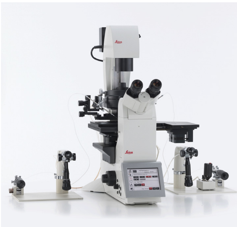
The perfect ICSI workstation: Leica DMi8, 3-plate stage, condenser S40 for modulation contrast for objectives 5x to 63x, new Narishige manipulators with injection units, heating stage 37°C.
