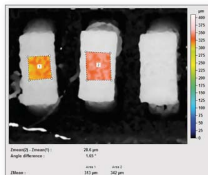
Coplanarity of contact zones on an electronic component using the step height (surfaces) study
