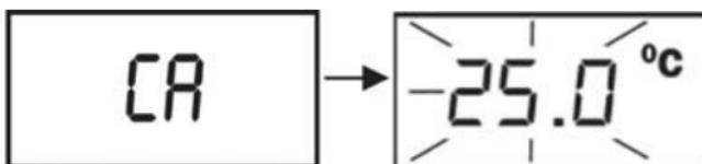
3 Compare the measured value of the temperature probe with the reference thermometer. Use **MODE/INC** to adjust the reading to the desired value. The maximum adjustment is  $\pm 5^{\circ}\text{C}$ .
