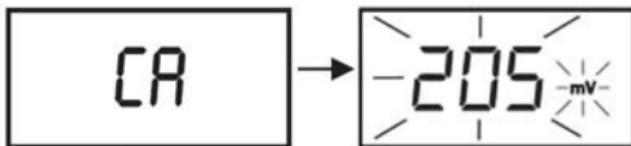
3 Use **MODE/INC** to adjust the reading to the desired value. The maximum adjustment is  $\pm 50$  mV.
