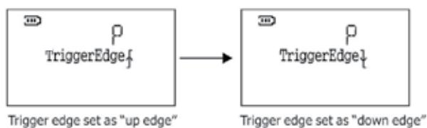
When trigger edge setting is set to “up edge”. The flash will occur on the leading edge of the input pulse (when delay setting is zero).
