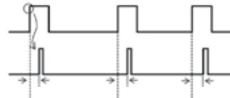
When trigger edge setting is set to “down edge”. The flash will occur on the trailing edge of the input pulse (when delay setting is zero).
