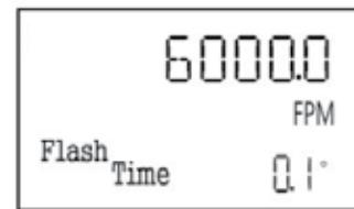
To set the flash pulse duration while in the modifiable mode; press "+" key, or turn the dial in the clockwise direction to increase the flash pulse duration by 0.1° increments.
