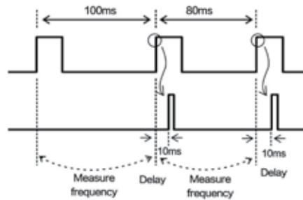
If the period of the external input is less than the setting of the delay time, the delay time is ignored and the ST-329BL flashes as if the delayed time equals 0.
