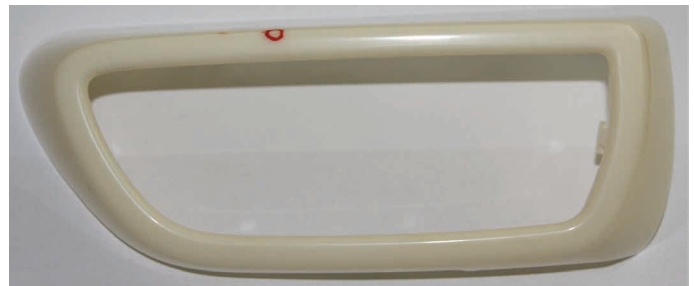
Side view of the air outlet cover panel (red circles mark defects)
