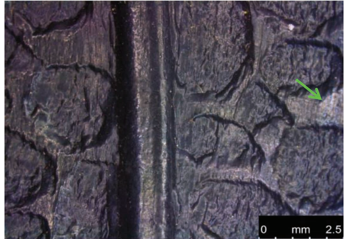
Automobile tire, tilt angle 15^\circ : more fine details visible on the black rubber surface with tilted view
