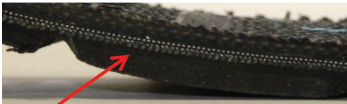
Cross section (red arrow) of the automobile tire sample with inner wall surface above
