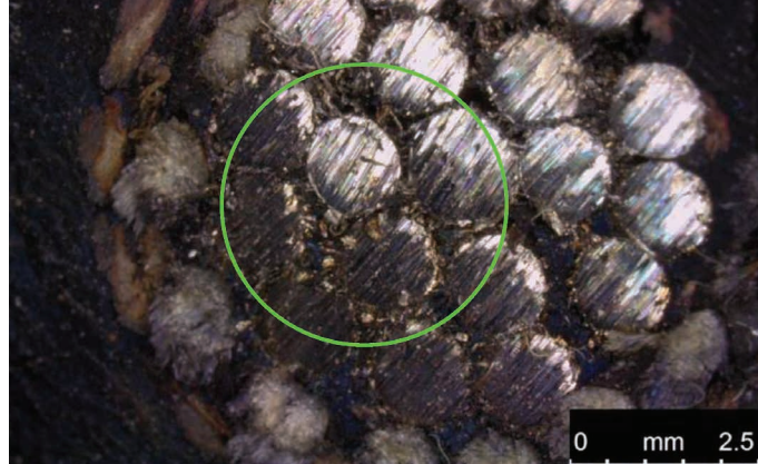
Full ring light illumination of automobile tire cross section: center features highlighted due to back reflection
