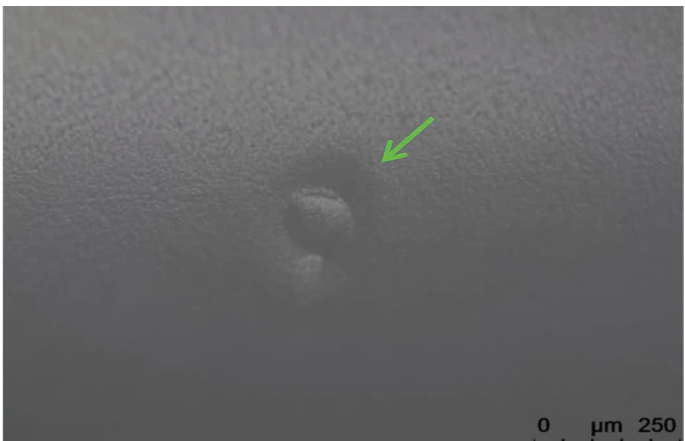
Quarter ring light illumination of the same air outlet panel shown above: better contrast for surface flaws
